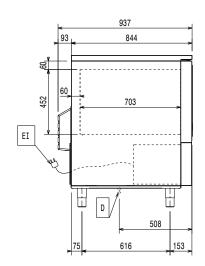
Drain Electrical inlet (power)
